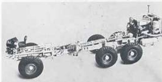
Reynolds Boughton "Griffin" 6 x 6 chassis G.V.W. 38 ton
