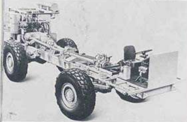
Reynolds Boughton "Phoenix" 4 x 4 chassis G.V.W. 25-26 ton
