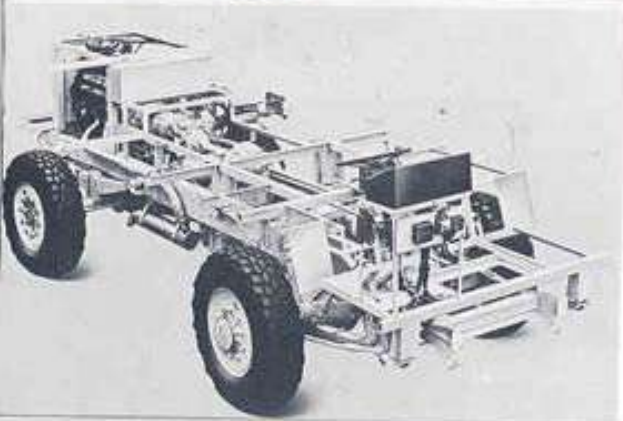
Reynolds Boughton "Pegasus" 4 x 4 chassis G.V.W. 7 tons
